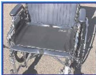
When the wheelchair Pressure PAD is installed it can detect the availability of a wheelchair based upon the activation of the Pressure PAD. Once activated the Pressure PAD transmits to the PalTrack RTLS system both the location of the wheelchair and if it is occupied or not. This information is displayed on the PalTrack computer screen and provides a quick assessment of the status of the wheelchair.
