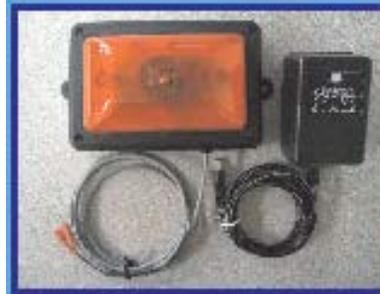
The Audio Visual Module (AVM) is a comprehensive alarming device that can produce a visual and/or audible notification. The AVM is designed to accept either normally opened or normally closed dry contact closures. The AVM is a self-contained unit with its own wall-mounted power pack.
