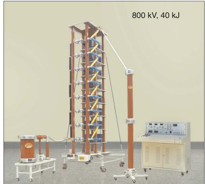
The Impulse Generator is an apparatus which produces very short high voltage or high current surges. High impulse voltages are used to test the strength of electric power equipment like insulators, Lightning arresters, alternators, instrument transformers, high voltage cables, power transformers, condenser bushings etc., as per relevant national and international standards.
